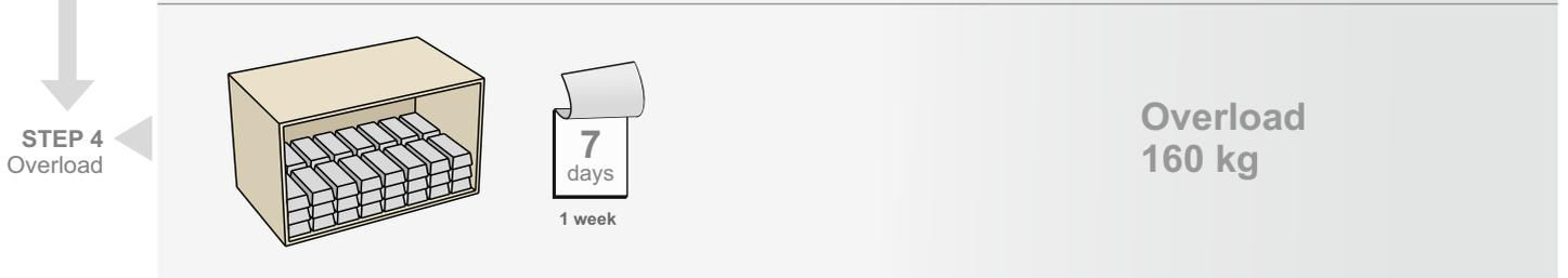
At the end of the tests the hangers and all cabinet parts are not damaged.
