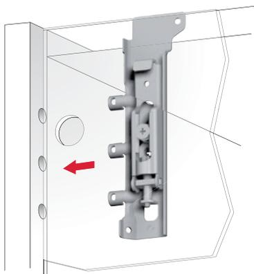
recommended fixing countersunk head wood screws  $\varnothing$  3,5x20 mm
