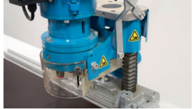
Fig. 4: Sliding guard at drilling spindles
