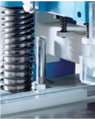
Fig. 14: Setting drilling depth
